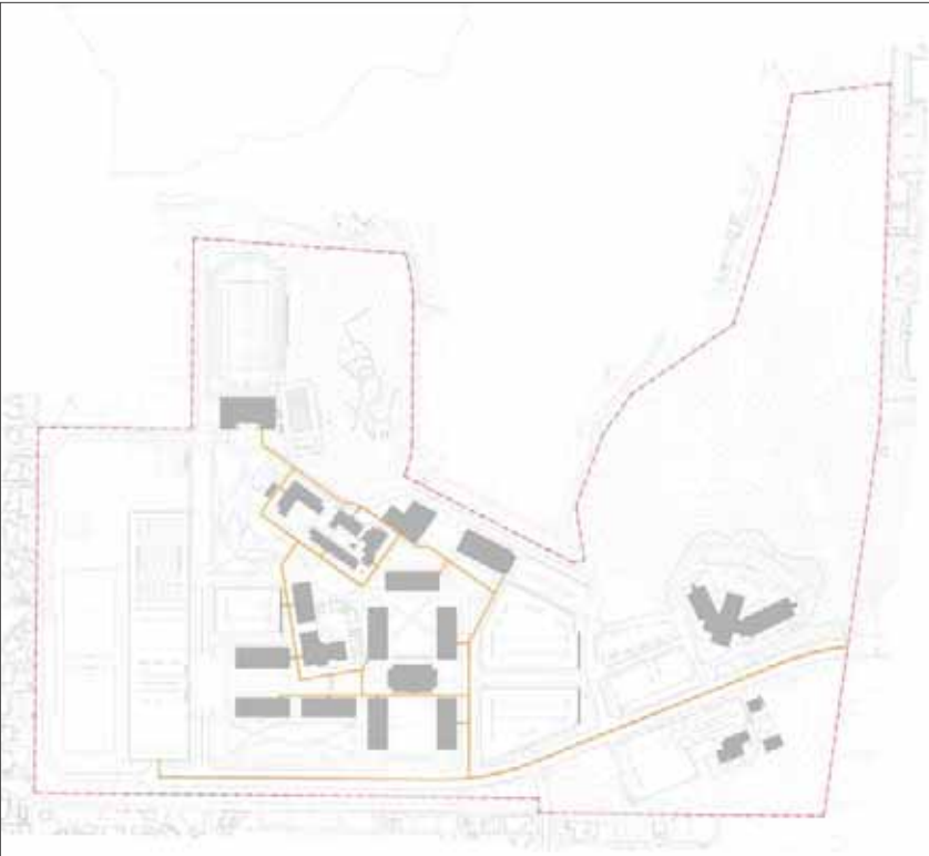
Domestic Water Distribution in the 16,000 Student Plan
