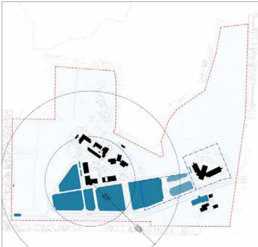
Parking Diagram "A": Existing Facilities. This diagram shows all existing parking on campus including the two lots on the John F Kennedy High School property. Including the high school parking +/- 2,100 spaces are accommodated on campus in about 17 acres. Without the 300 spaces on high school property east of Campus Drive approximately 1,800 spaces are available to the campus. At a ratio of 1 space for every five students this inventory supports a student population of 9,000.
