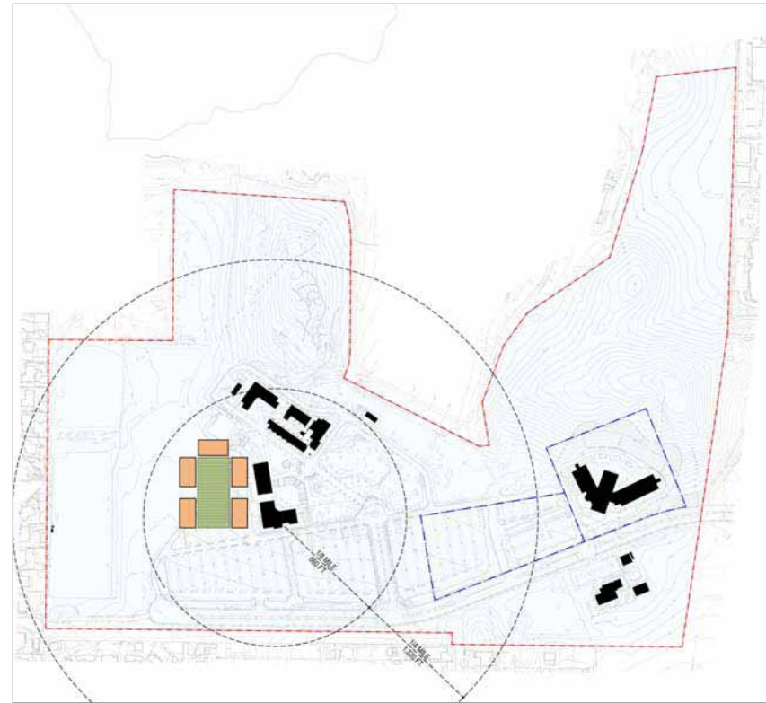
Buildings and Open Space Diagram "B": 10,000 Students. This diagram shows approximately 160,000 SF in five new buildings, 32,000 SF each in double loaded two story formats that would on a rough order of magnitude be required to support a student population of 10,000.
