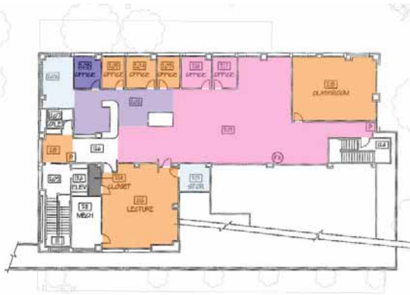
Student Services Second Floor. Rooms color coded by taxonomy of program (TOP) code designation.
