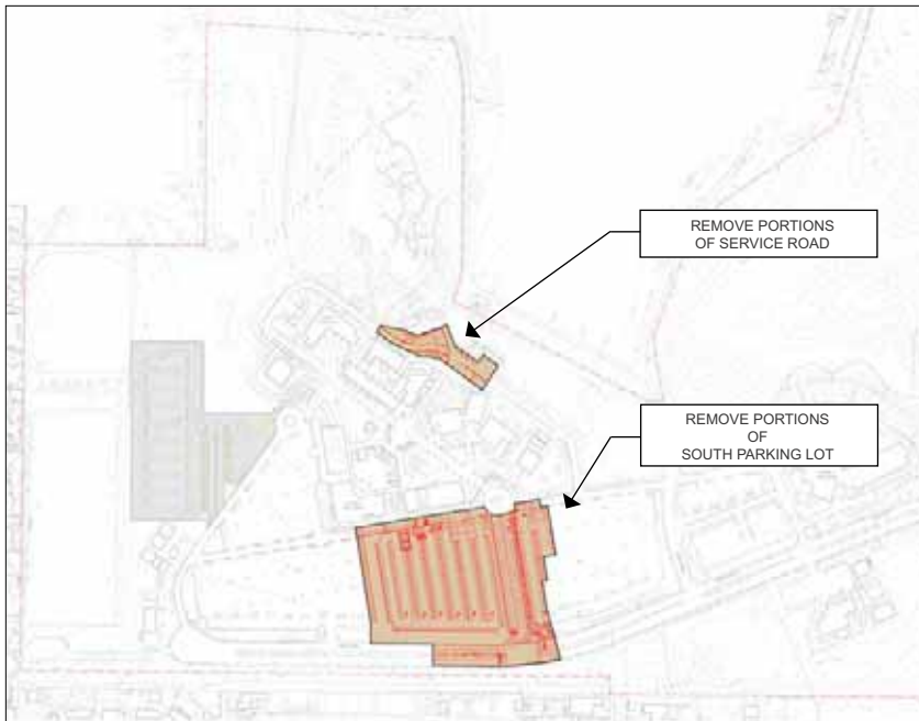
Demolition of Parts of South Parking Lot and North Mesa Service Road.
