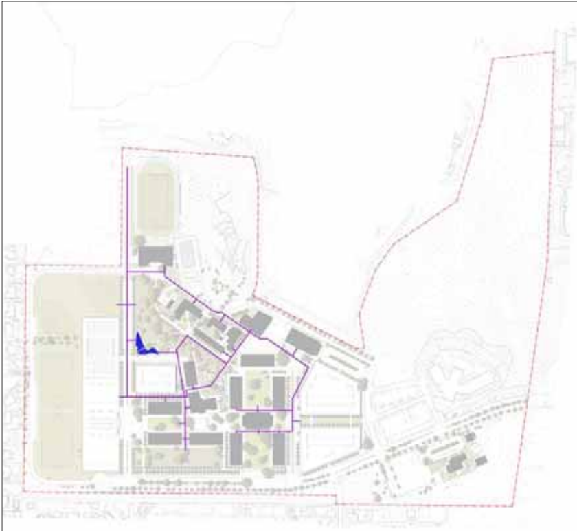
Reclaimed Water Distribution in the 16,000 Student Plan
