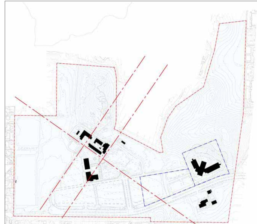
Geometry “A”: In Alignment with the Central Promenade and North Buildings of the Mesa. The buildings at the far north side of the mesa are oriented in a SW-NE alignment roughly parallel to the slope of the natural topography. Extending this geometry south and east toward 3rd Street would create awkward intersections and inefficient shapes for parking lots at the perimeter of campus
