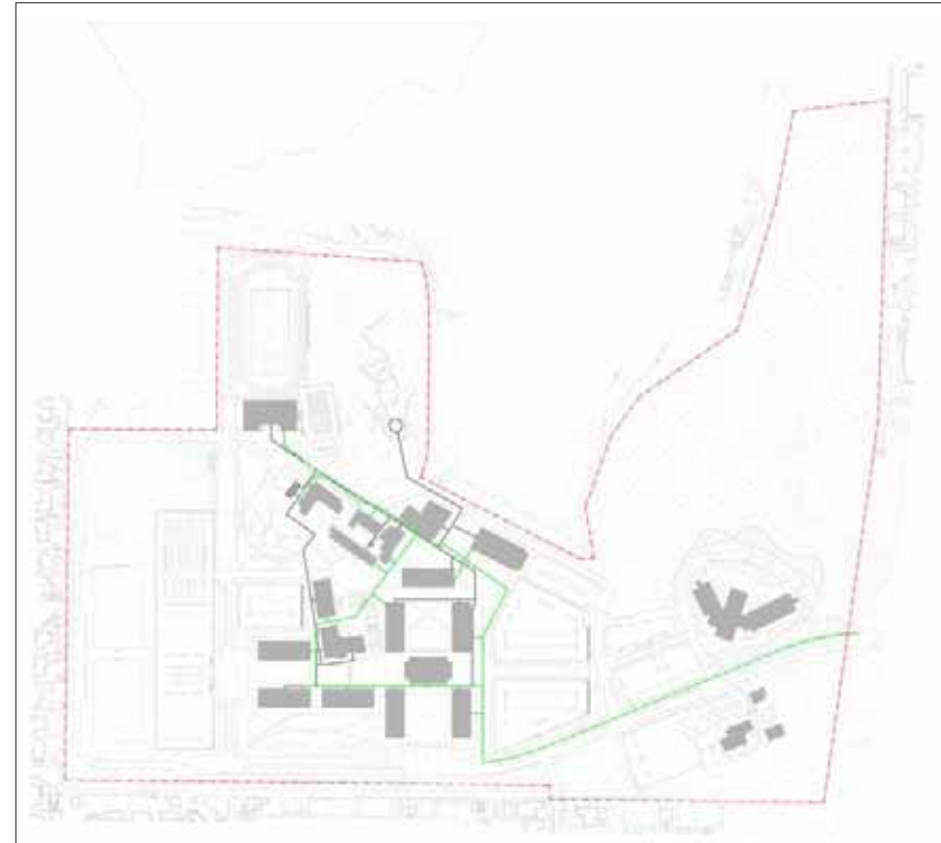
Gas and Mechanical Distribution in the 16,000 Student Plan
