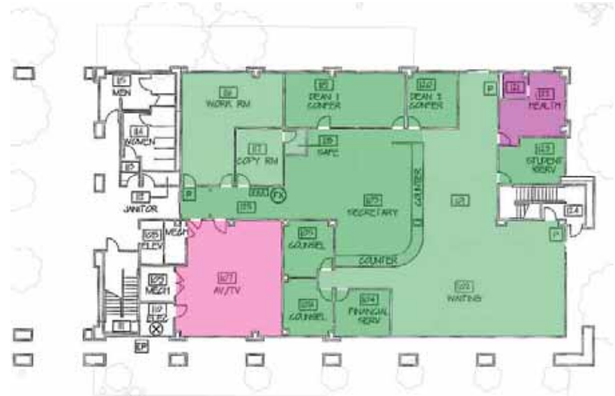
Student Services First Floor. Rooms color coded by room use type designation.
