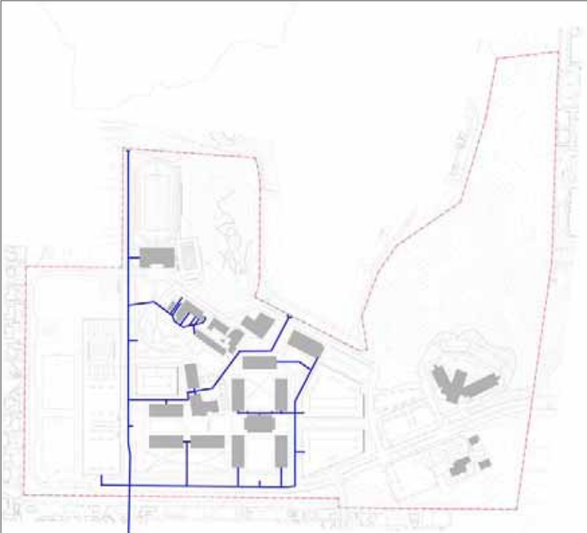
Storm Water Drainage in the 16,000 Student Plan
