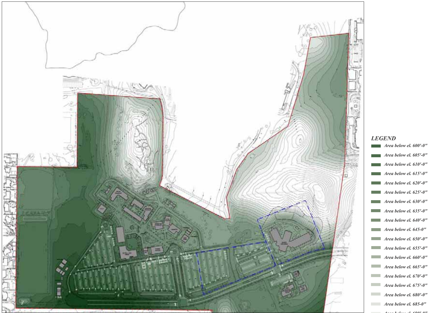
Topographical Profile of the Existing Norco Campus. Most of the core campus sits on gently sloping land. Steep hillsides form the north boundary of the core campus, one just north of the Applied Technology Building, the other north of John F. Kennedy High School.
