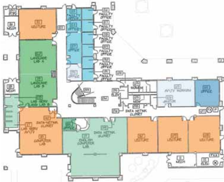
Library Ground Floor. Rooms color coded by taxonomy of program use (TOP) designation.
