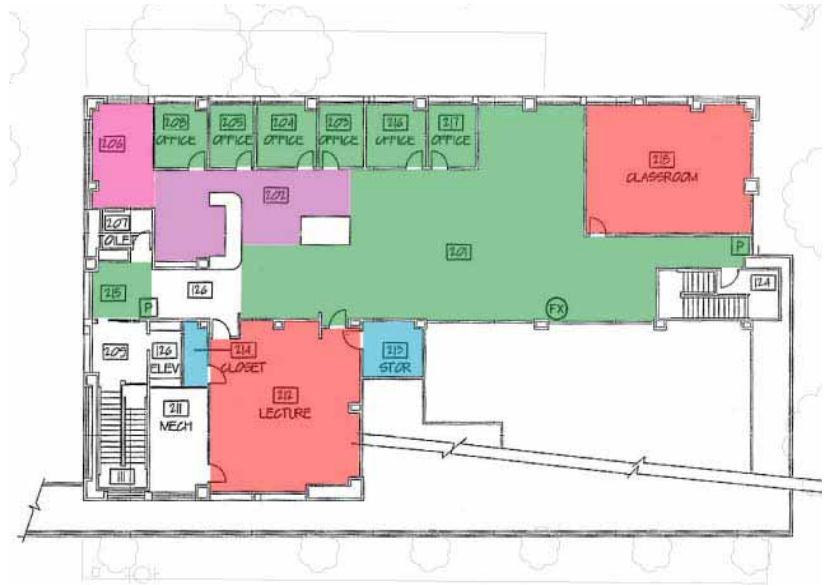
Student Services Second Floor. Rooms color coded by room use type designation.
