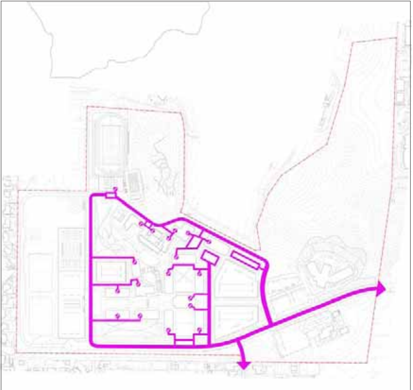
Waste and Recycling Vehicle Access and Circulation
